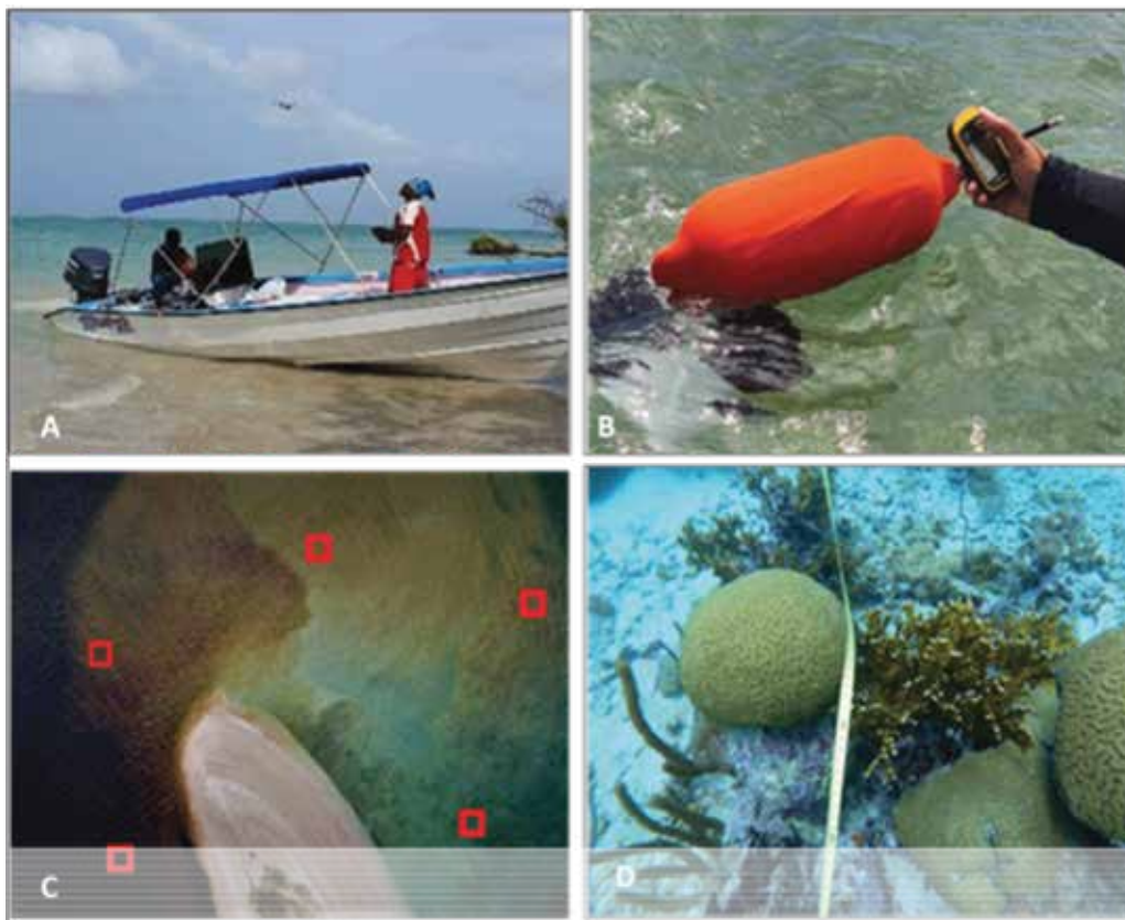
Figure 2. UAV launch from Vessel (A), deployment of Ground Control Points and georeferencing (B), GCPs at study site (marked by red squares) adapted from drone footage (C) and underwater transects for benthic surveys (D).
